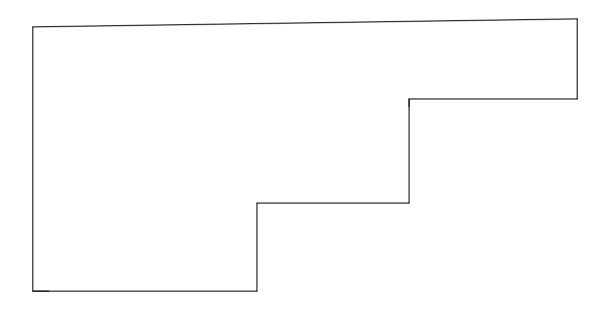
The largest portion of the structure that can be divided into a perfect rectangle is the western half. It would be most efficient to start in the southwest corner working north from left to right. The cut end at the end of the first row will be used to begin the next row.
