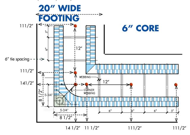
**Note:** The use of two corner pins is not required but helps in setting the rebar into the proper position when the block is not wet-set. If using outer corner pins for the stem only, you can eliminate them in the upper walls and use the corner web placement point only.
