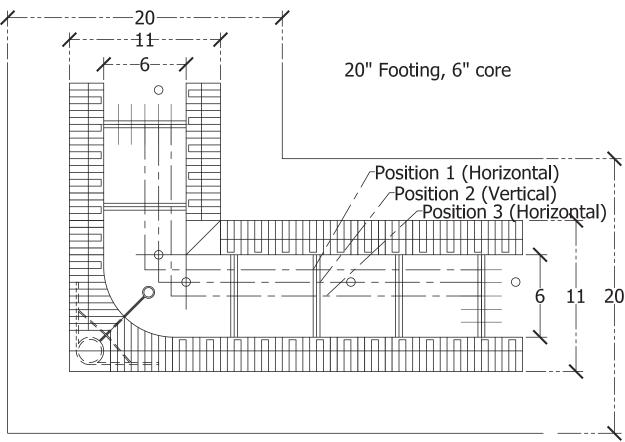
Alignment Shown: Below Grade (Tension Side) Above Grade alignment - Centerline of Form.
