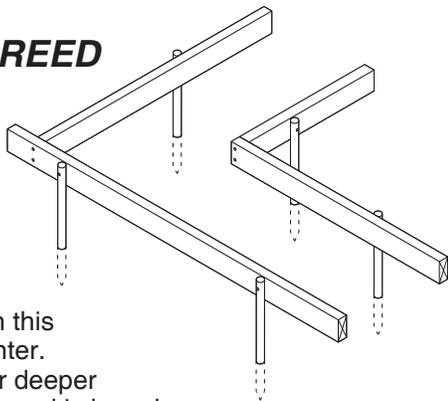
Drive the stakes on this line about 6' on center. Reduce spacing for deeper footings or if the ground is less dense.
