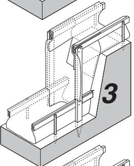
Screw plywood bulkhead in position and brace as required.
