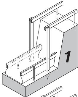
Run fabric up bank to form step. Most steps are too deep to form with a single fabric width. Either run two widths of fabric as edging or turn the fabric 90 degrees to obtain the required width.
