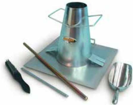
Concrete Slump cone
