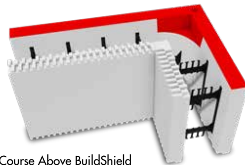
Figure 2.2 Corner form modified to remove foam radius in corner for BuildShield installation. Note radius is only removed to a depth of 3". Corner form modified to remove interlock fingers and foam radius removed in corner for BuildShield installation. Note this form is placed with the modifications toward the BuildShield Extrusion Track.
