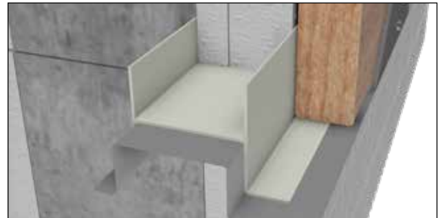
The BuildShield stainless steel barrier wraps around the extrusion track. The stainless steel barrier extends under the edge of the rim joist. Screw from the underside every 12" to ensure stainless steel barrier remains in place during a fire.
