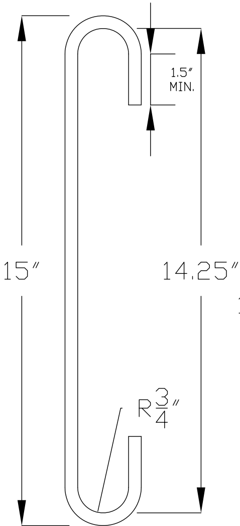
RECOMMENDED STIRRUP FOR BD-1200+4" RISER
