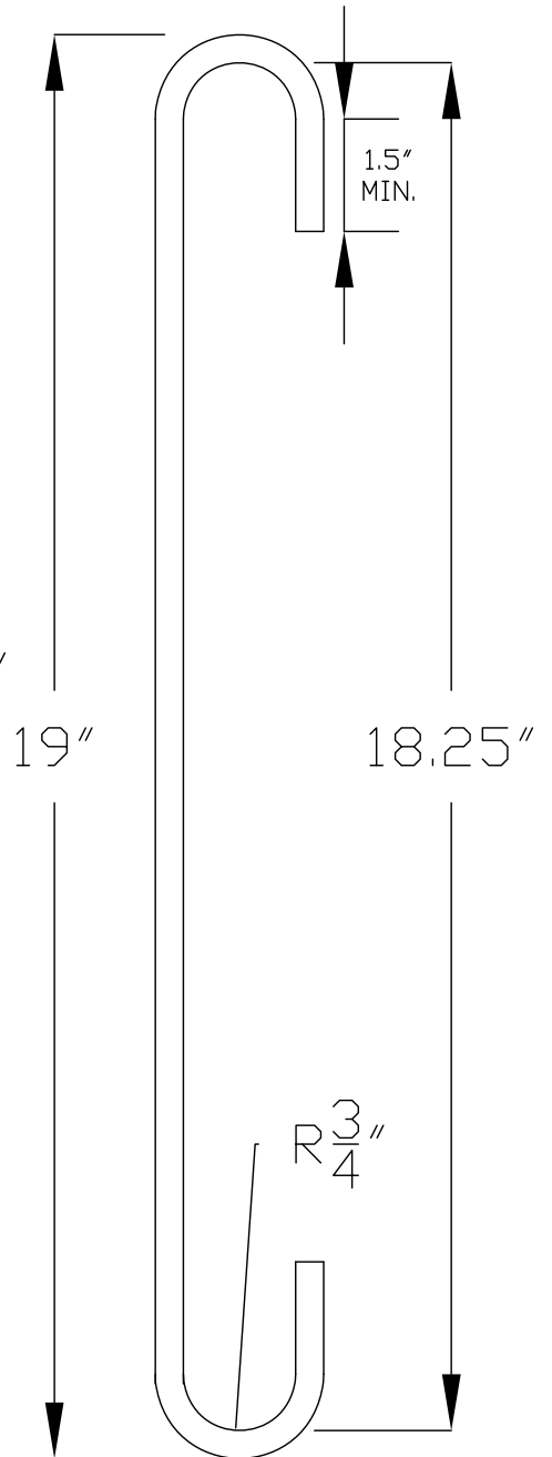
RECOMMENDED STIRRUP FOR BD-1200+8" RISER
