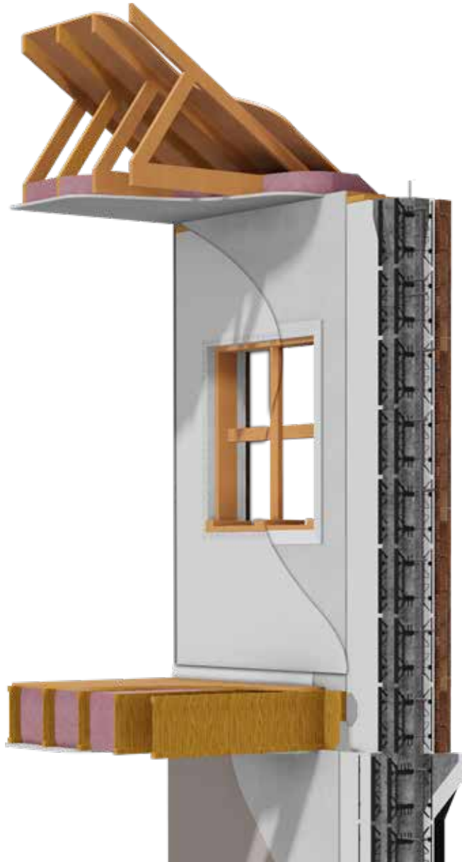
Figure 1.4 BuildBlock basement and first floor showing cutaway of BuildBuck integrated into wall with cross bracing.
