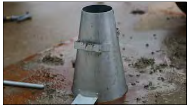
Concrete Slump cone
