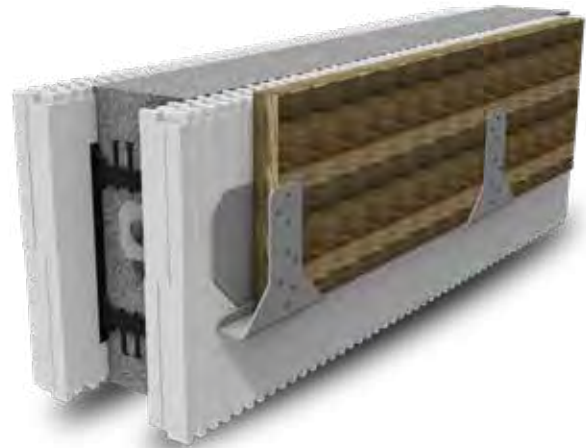
Figure 5.10.3 Steel bearing plate embedded into the top of an ICF wall. Ensure the correct height taking into account the interlock.
