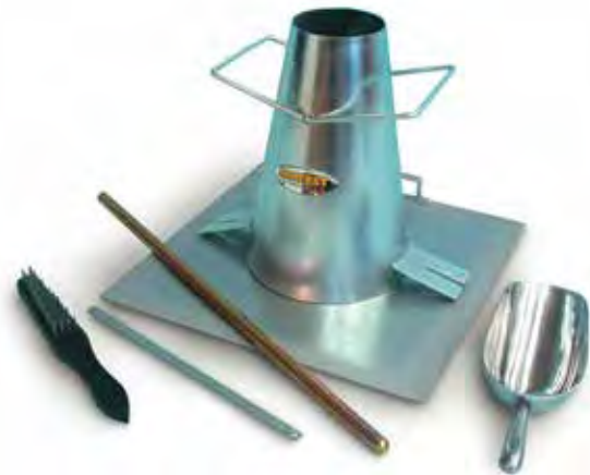
Concrete Slump cone
