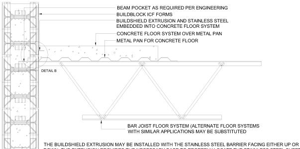
DOWN. THE EXTRUSION PROVIDES THE NECESSARY BASE TO PROPERLY LOCATE THE STAINLESS STEEL SHEET MATERIAL DURING ALL PHASES OF CONSTRUCTION.
