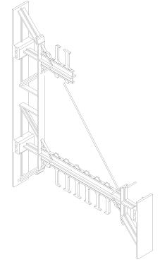
BUILDCLIP IS OFFERED FOR 6" AND 8" BUILDBLOCK FORMS. BUILDCLIP WILL NOT WORK WITH BUILDBLOCK KNOCKDOWN FORMS. BUILDBLOCK RECOMMENDS BUILDBLOCK 6" FORMS MINIMUM WHEN USING BUILDDECK ICF FLOOR AND ROOF PANELS.
